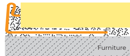
Cross-sectional image of a Schlüter®-Schiene-E profile
