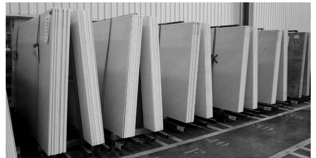
Storage of Neolith slabs in the shop
